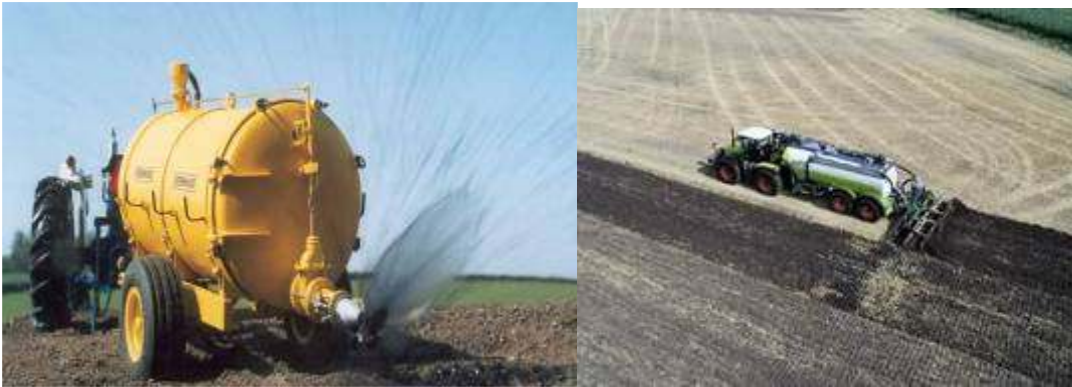
Plate 1.17: Typical heavy slurry tankers, expensive and the cause of soil compaction
