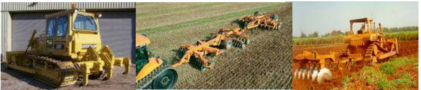
Plate 1.3: (from left to right) Cat ripper equipment, heavy discing equipment and light discing/ finishing equipment
