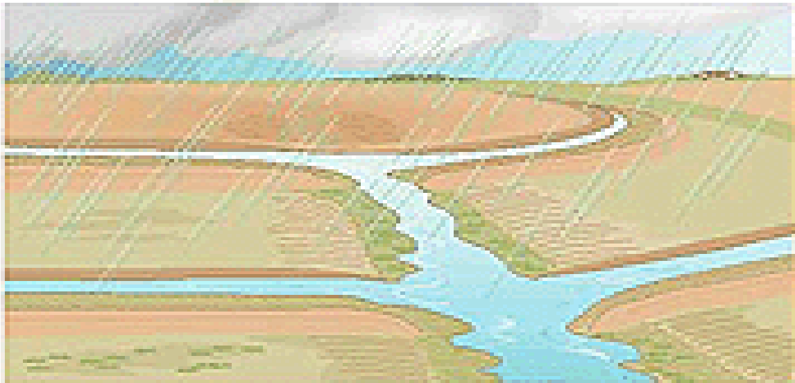
Figure 1.7: Illustration showing contours discharging into grassed waterways
