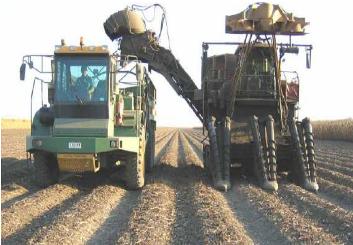
Plate 1.5: An example of controlled traffic. The machinery only passes in the inter row area, leaving the growth zone intact.
